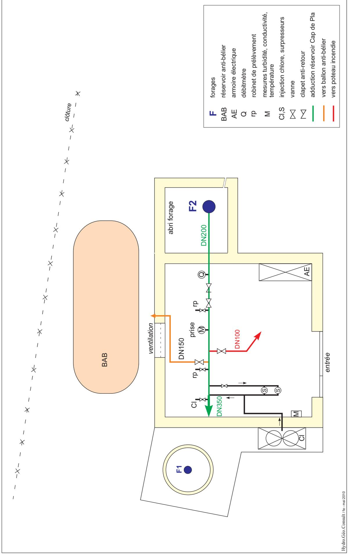
Figure 5 - CONSTRUCTION FORAGE F2 PLATE-FORME DU RATIER A NARBONNE
